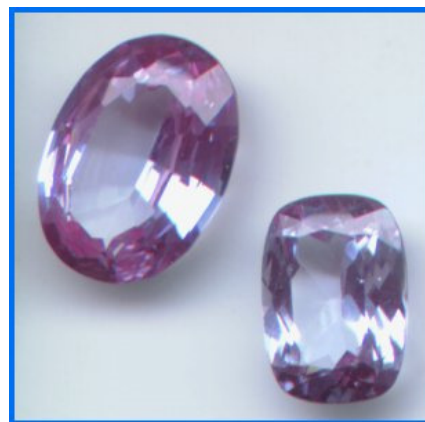
Synthetic spinel aquamarine substitutes. Purplish hue results from selective absorption and transmission of light.
