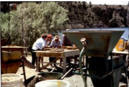
Mechanical shake table used to separate high specific gravity mineral that may contain sapphires.
