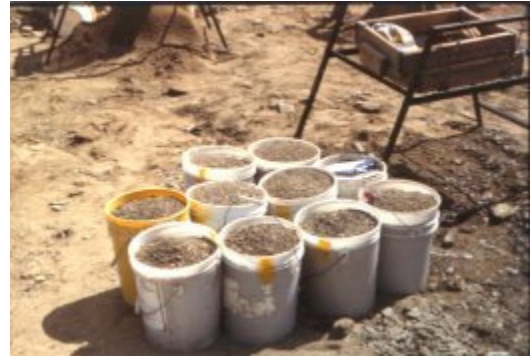
Sized and sorted gravel concentrate that may contain sapphires. Note manually operated sieve at back.
