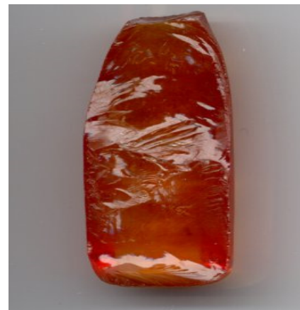
Boule of synthetic sapphire. Boules develop split upon cooling.
